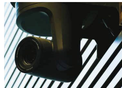
Panasonic AW-HE120 PTZ cameras are fed to an AW-RP50 controller
