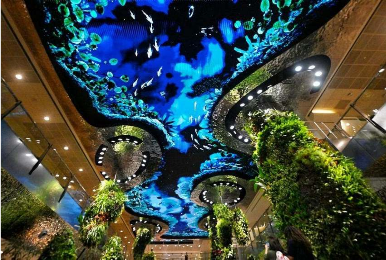
Like a skylight, the digital sky emulates daylight and meteorological conditions in real time through integration with the airport weather system. ST PHOTO: KUA CHEE SIONG
