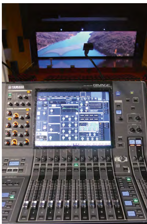
A Yamaha Rivage PM5 has been installed in the main auditorium control room
